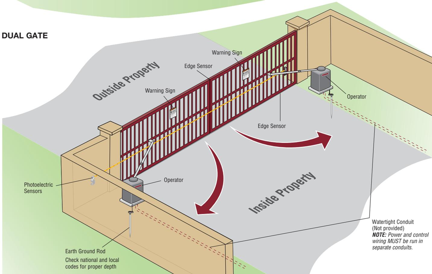
**NOTE:** Power and control wiring **MUST** be run in separate conduits.
