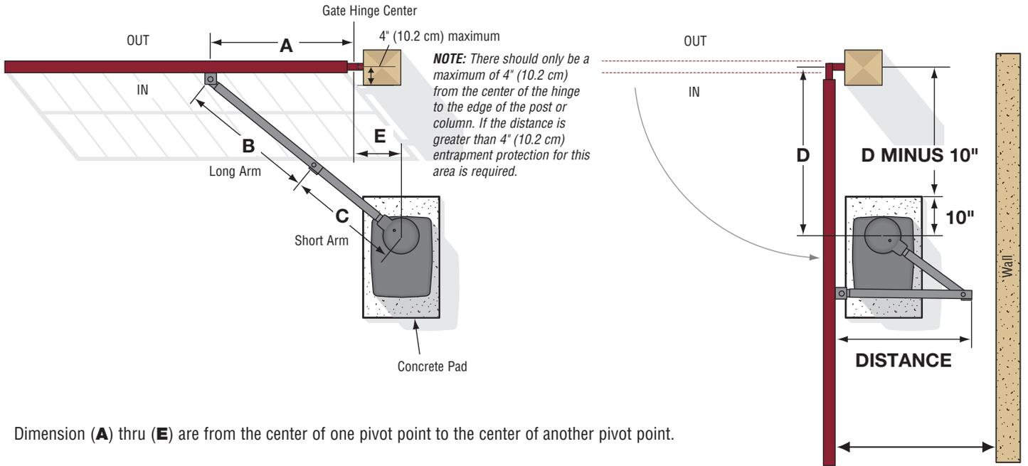
Dimension (A) thru (E) are from the center of one pivot point to the center of another pivot point.
