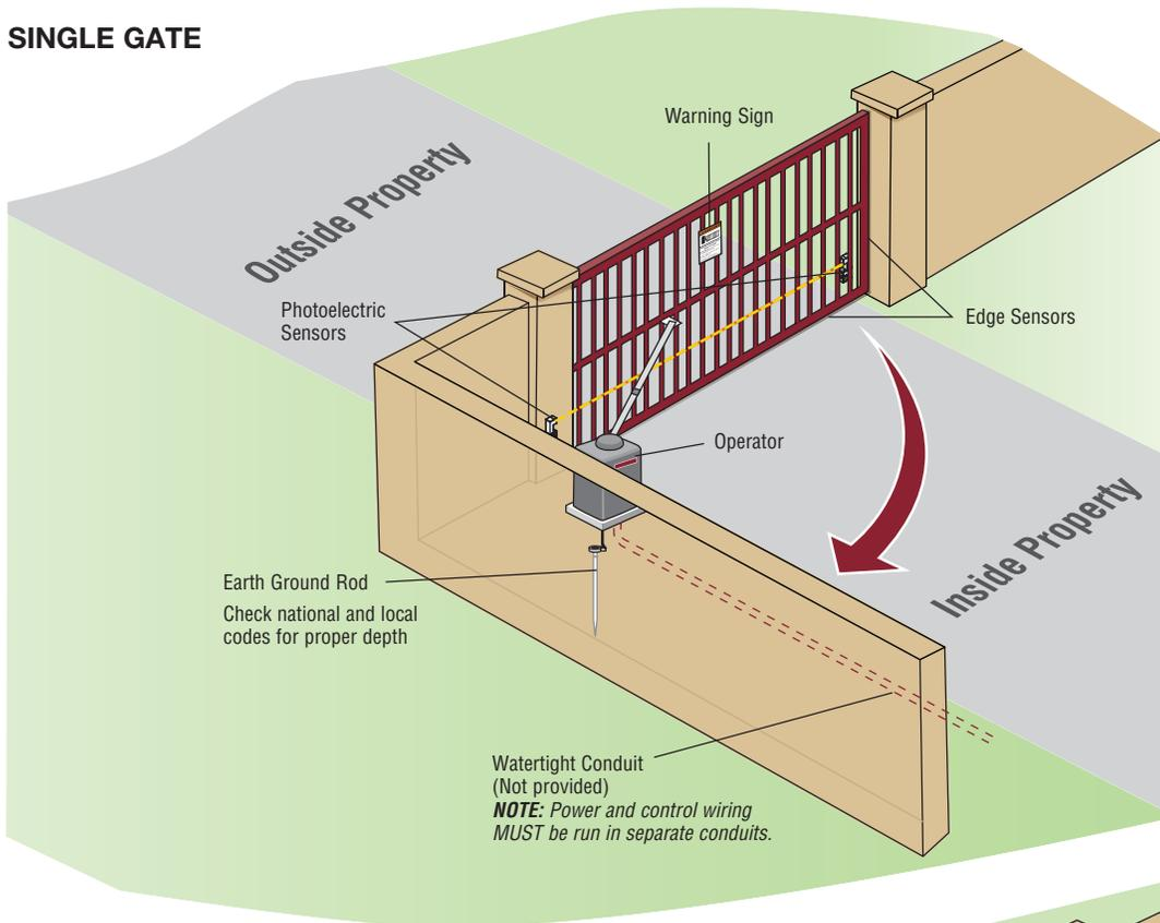
**NOTE:** One or more non-contact sensors shall be located where the risk of entrapment or obstruction exists at either the opening or closing direction. Care shall be exercised to reduce the risk of nuisance tripping, such as when a vehicle, trips the sensor while the gate is still moving.
